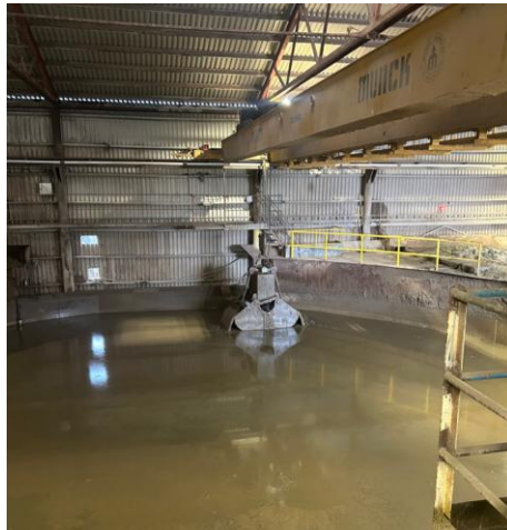
Extraction from “Cuttings Pit”
