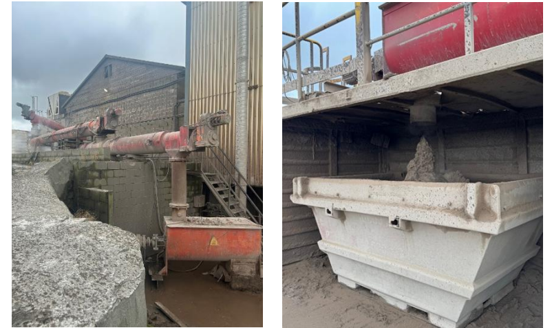
Processed Dried Cuttings Transported to Skips
